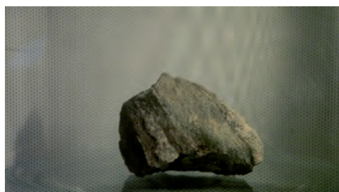
Performance of Olkiluoto Mica Gneiss in Microwave, 700 Watt, 1'58"
